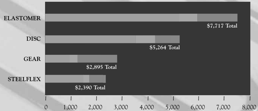
Coupling Lifetime Operating Costs 150 HP (112 KW) @ 68 RPM
