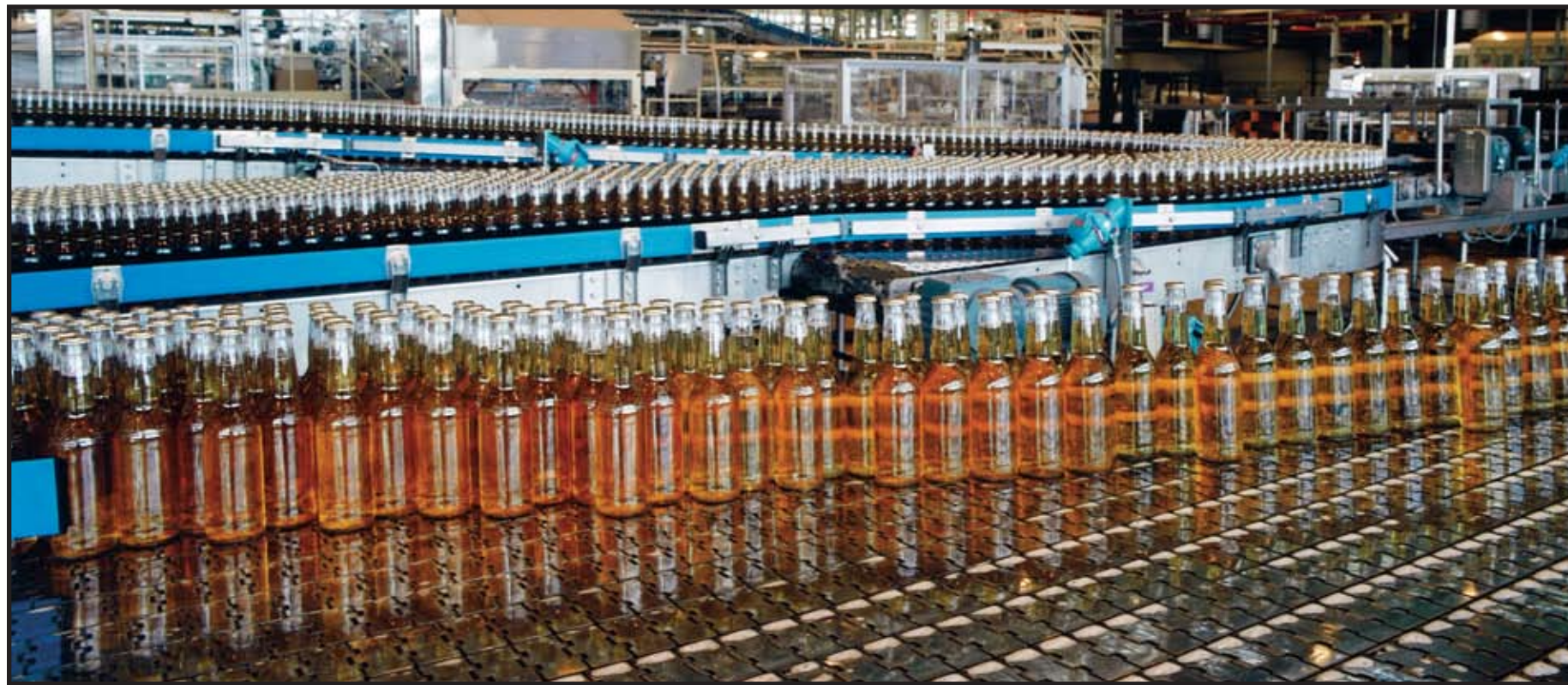
New Rexnord X-Line Series steel chains at a brewery inliner
