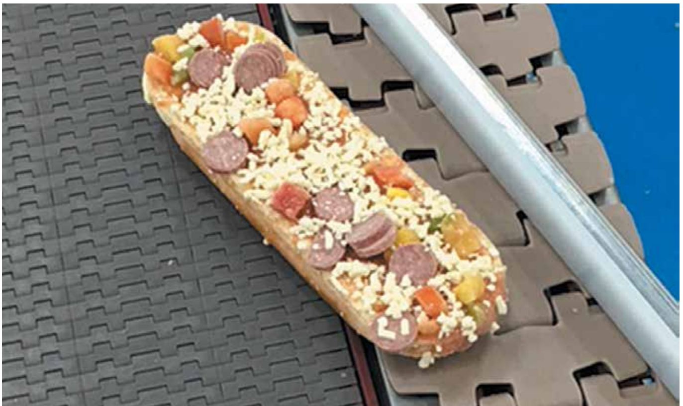
Conveyor equipped with Rexnord 395 Series KleanTop Belt.
