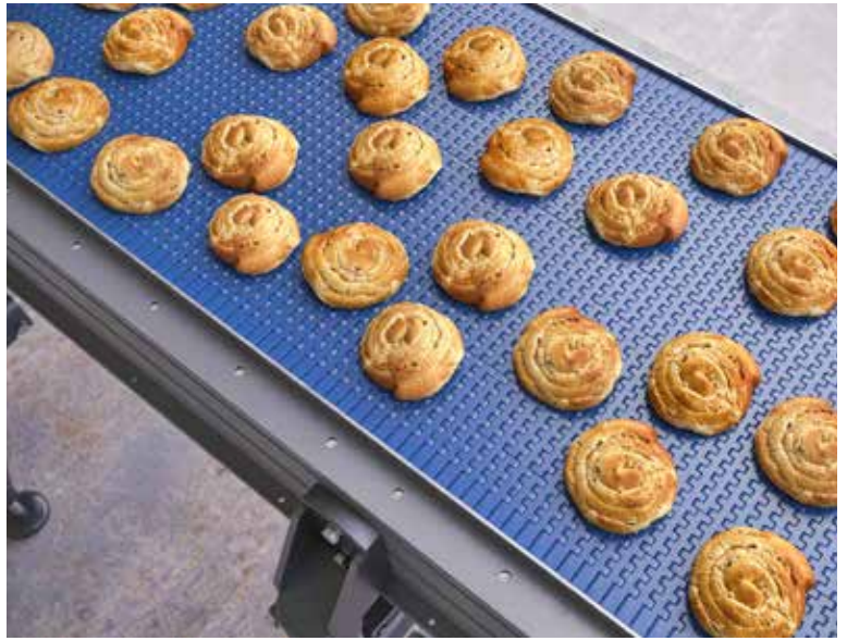
Conveyor equipped with Rexnord 595 Series KleanTop Belt.
