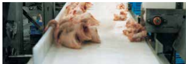
Chicken deboning line with 2015 mattop chain
