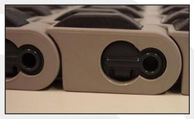
A new special clip has been designed, to retain the metal rods of the TCF-belt. The clips are flush with the edge of the belt and not exposed at the top surface of the belt. The new clip closes the hinge eye completely, offering a secure lock. The clip can be operated from the side and from below and can be re-used.
